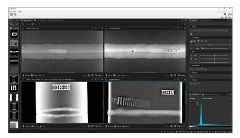
D-Tect X provides an optimal and time-saving NDT inspection workflow: from image acquisition, image evaluation and report generation to data import and export, everything you need is included.
