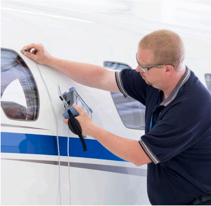
Resonance mode configured as "go/no-go".
