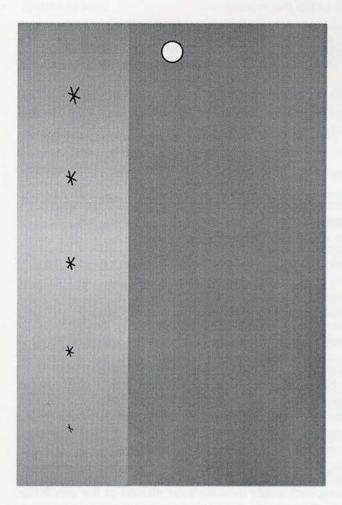
The Sherwin PSM-5 panel, a "known defect standard," is the most practical means to meet the MIL-STD-6866 and ASTM E-1417 requirement for a <u>daily system performance check</u>. It also conforms to the P&WA TAM 146040 specification, and meets other company specifications as well.
