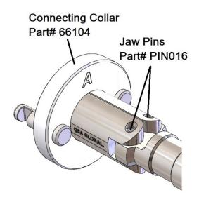
4.4.22 Replace any damaged, bent, or loose-fitting jaw pins **(PIN016)** by installing new pins in the larger side of the jaw hole until a 3/16-inch drift punch has bottomed, which will automatically center the pin.
