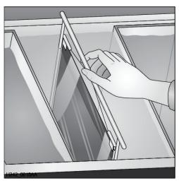
Place the film in the stop bath for 30 seconds. Agitating moderately, lift from the stop bath and drain well.
