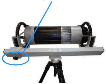
After loading and adjustment of the arm, the tube head should be locked by means of the two clamps located in each end of the cradle
