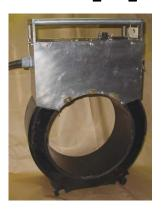
The WDV-10 shown here, has been in field service for 2 years, and was equipped with ID Wear Bars prior to being delivered to the customer. ID Wear Bars are made of Brass, so they won't damage the part under test, and will slide easily on the workpiece.
