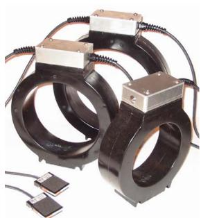
Western's new WA-Series of AC Coils are the most powerful Portable AC Coils in the inspection World. All 4 models are rated at over 4000 Amp Turns at 115VAC / 60Hz, and in excess of 5000 Amp Turns at 230VAC / 50Hz ("K" Models). The new WA-Series Coils have ID sizes that correspond to the model number; WA-8, WA-10, WA-12, and WA-14, with diameters of 203mm (8"), 254 (10"), 305mm (12"), and 356mm (14"). These 4 new models replaced our dated WAC-10.
