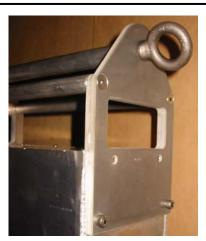
WDV-16 and larger Coils are a little heavy to be handled by a single operator, so Western has designed a Vertical Lifting Lug assembly that is attached to the Control Housing. This feature allows the Coils to be lifted (or suspended) vertically, for convenient positioning on and off of the workpiece. If horizontal handling is required, Western can also provide the Lower Lifting
