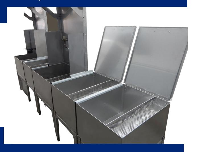
Station 10: Tunneltype swirl cloud developer with automated controls, HEPA certified dust collector. 120VAC.
