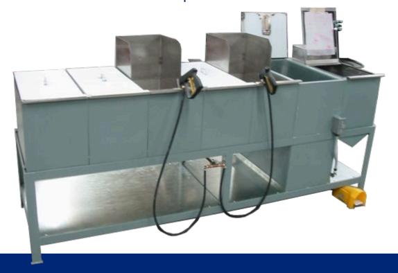
**Station 5:** Final rinse tank with rigid backsplash, hose, and spray nozzle.
