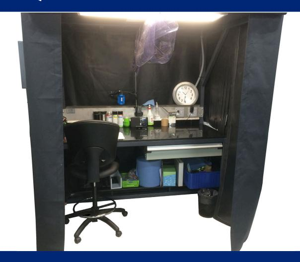
Station 4: Electronically heated, thermostat controlled dryer. Black front curtain, fire resistant and penetrant resistant. Made of 304 stainless.
