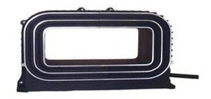
These demagnetizers have field strengths that range from 210 to 420 gauss. They are designed to operate in a continuous [C] or intermittent [I] mode in a dry environment. Units are available for operation on 120, 240, 480 or 575 volts, 50 Hz or 60Hz, single-phase power. Intermittent types are rated for 25% duty with a maximum 'ON' time of 5 minutes. Units may be sealed for operation in 'nondry' conditions.
