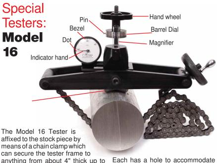
The measuring head is independent of the clamp and may be removed for mounting on a holder of your own design.
