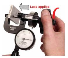
Shown here is a major load of 150 kg being applied for reading in the Rockwell C scale. With Ames Superficial tester models, the gauge shows 15, 30 and 45 kg pressures and indicates in the Rockwell N and T scales.
