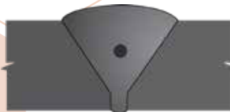
34 Single Gas Pore in Single Vee UT, RT
