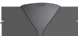
20 Crater Crack (crown stop-start area) MT/PT, UT
