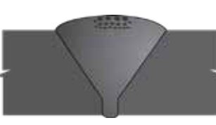
32 Porosity in Single Vee (surface breaking) VT, MT/PT
