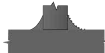
91 Weld Splatter on Filler VT, RT
