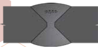
30 Porosity in Double Vee (sub-surface) UT, RT
