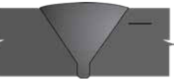
50 Lamination in Single Vee (base metal) UT
