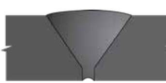
70 Root Concavity in Single Vee VT, RT
