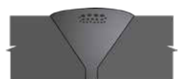
30 Porosity in Single Vee (sub-surface) UT, RT
