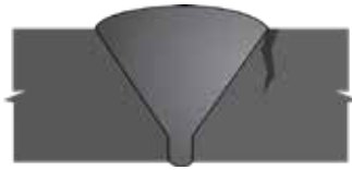
10 Toe Crack in Single Vee MT/PT, UT
