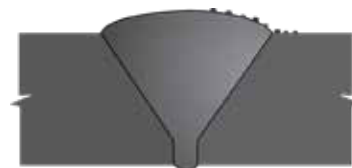
90 Weld Splatter on Single Vee, VT, RT
