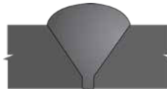
74 Excess Crown in Single Vee, VT
