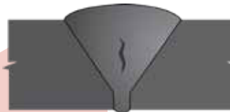
15 Centerline Crack, Single Vee (sub-surface) UT, RT
