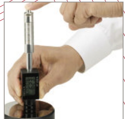
3. Place it on the material to be tested and push the button.
